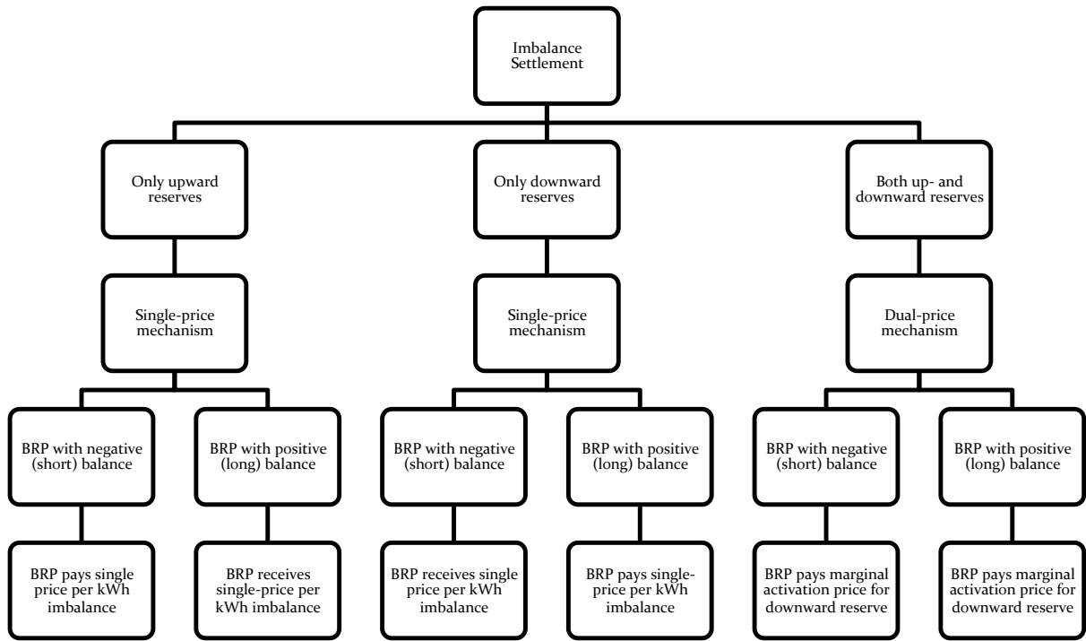
Figure 3: Imbalance settlement in the Netherlands, combination of single and dual pricing ([14], p.191)
